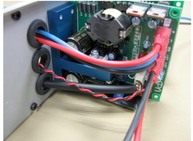
Reverse the bridge. Strip the blue / black wire for about 2mm and connect them as shown right. Use the following connections:
