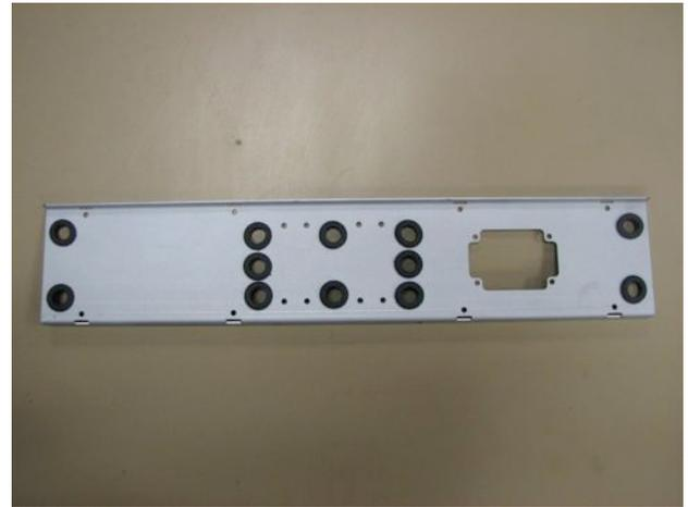
Mount 4 studs (M3\*6) using 4 bolts M\*6, all from bag #1.
