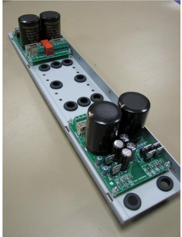
Mount both UCD modules to the bridge, mirror matched. The result should look like shown right. Use 8 pieces M3\*6 bolts. Tighten these well.
