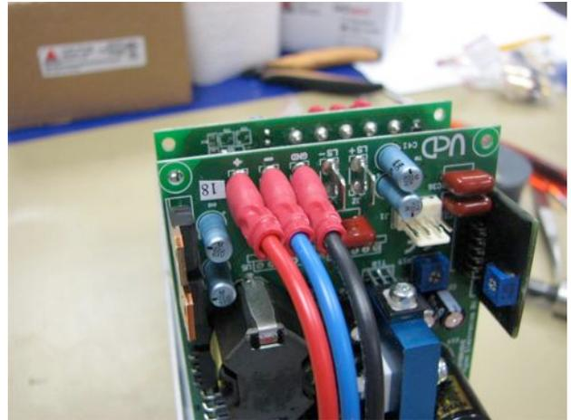
Once that is done, fix the speaker wiring, at the same side of the UCD modules. Use:
